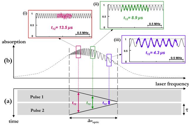
Fig. 2. (Color online) (a) frequency chirps during engraving; (b) schematic absorption profile, *dashed and solid line*: without and with engraving; (i)–(iii) normalized experimental transmission spectra and sinusoidal fit. The maximum contrast reaches 15%.
