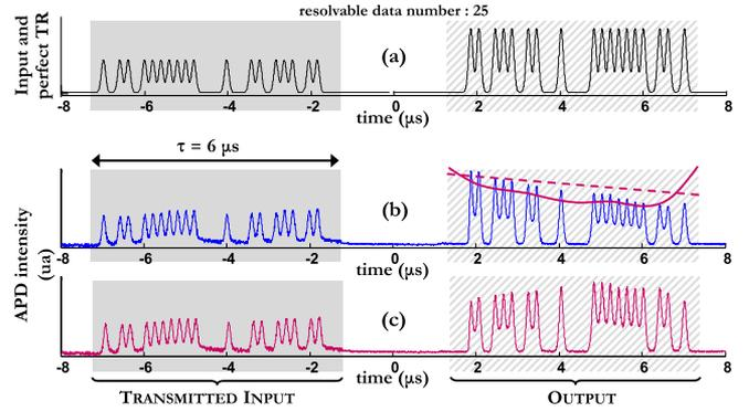
Fig. 3. (Color online) Input and output pulses: (a) input and perfectly time-reversed output; (b) single-shot experimental transmission, *dashed line*: effect of interaction of  $\text{Er}^{3+}$  with fluctuating environment, *solid line*: effect of optical depth variation over  $\Delta\nu_{\text{optic}}$ ; and (c) output corrected for the two previously cited effects.
