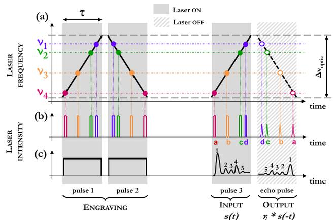
Fig. 1. (Color online) 3PE-scheme: (a) laser pulse (solid line) and echo (dashed line) chirped frequency, (b) 3PEs at four different frequency addresses, and (c) TR protocol: continuous engraving is achieved by pulses 1 and 2. The waveform, carried by pulse 3, is time reversed in the echo.
