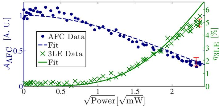
**Figure 3.** Two-level AFC echo area  $\mathcal{A}_{\text{AFC}}$  (dots) and three-level efficiency  $\eta_{3\text{LE}}$  (crosses) as a function of the square root of power of the control pulses. The dashed and solid lines represent a fit to the data as described in the text. Each data point is the average of ten trials. Error bars indicate the maximum standard error in the mean measured for each data set.
