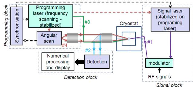
Fig. 2. Building blocks of the experimental set-up.
