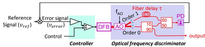
Fig. 3. Control and stabilization set-up of broadband arbitrary frequency sweeps. Abbreviations are defined in text.
