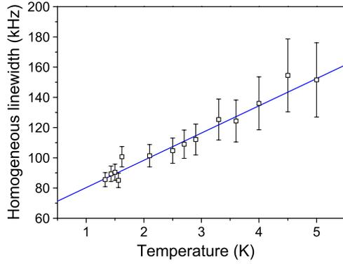
FIG. 3 (color online). Temperature dependence of the homogeneous linewidth  $\Gamma_h$  measured by two-pulse photon echoes. The solid line represents the linear fit to  $\Gamma_h = \Gamma_0 + RT$  with  $\Gamma_0 = 62 \pm 3$  kHz and  $R = 18 \pm 1.6$  kHz/K.
