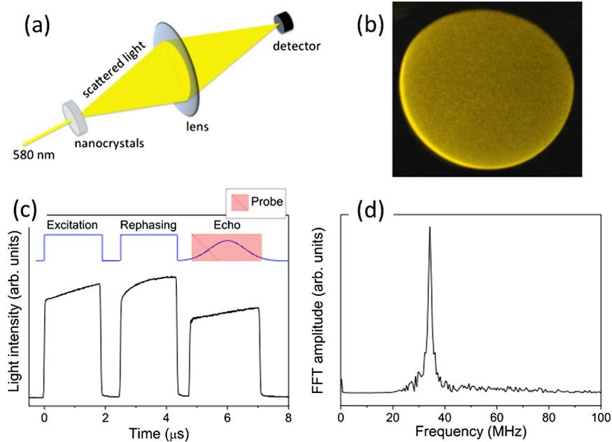
FIG. 1 (color online). Photon echo experiments on powders of nanocrystals. (a) Experimental scheme. (b) Speckle pattern observed for transmitted light through the powder. (c) Schematic two-pulse photon echo sequence (top, echo pulse not to scale) and corresponding signal (bottom). The probe pulse is shifted by 34 MHz for heterodyne detection. (d) Averaged fast Fourier transform (FFT) of the heterodyne detection beat signal after a 20 MHz cutoff high pass filter.
