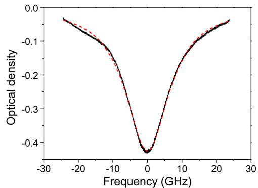
FIG. 2 (color online). Absorption spectrum of 0.86 at. %  $\text{Eu}^{3+}:\text{Y}_2\text{O}_3$  nanocrystals at 3.5 K (black solid line) and Lorentzian fit (red dashed line).
